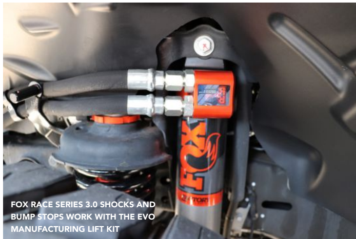
FINNED FOX REMOTE SHOCK RESERVOIRS DISSIPATE HEAT FOR MORE CONSISTENT DAMPING
