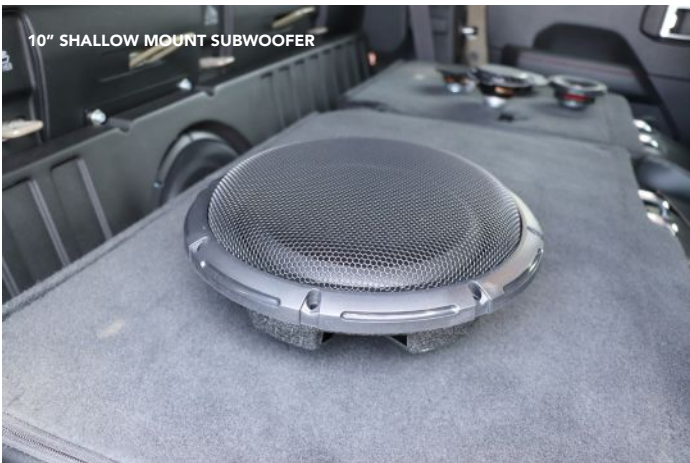
OEM AUDIO PLUS' 10" SUBWOOFER HAS A SEALED FIBERGLASS CABINET THAT USES LITTLE CARGO AREA
