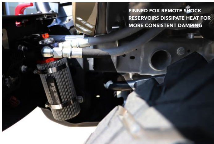
FOX RACE SERIES 3.0 SHOCKS AND BUMP STOPS WORK WITH THE EVO MANUFACTURING LIFT KIT
